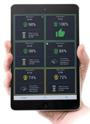
"The QCPR Training app is developed to support the cpr instructor. This is done via a bluetooth recording system and then this allows the learner to see the effective depth and rate of CPR compressions"
